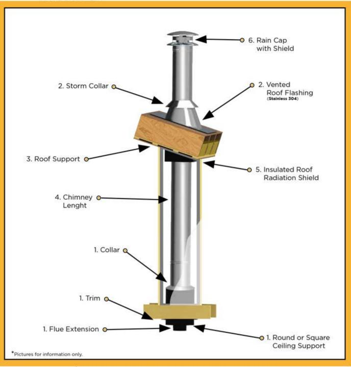
\*For installations that pass through an inhabited room, the chimney must be nested.
